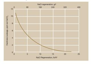
Capacity and Hardness Leakage graphs are shown assuming a service flow of 4 gpm/ft<sup>3</sup> (32 *Vh/l*) and total dissolved solids of 400 ppm and 20 grains of total hardness. The hardness leakage will increase and the capacity will decrease while increasing total dissolved solids and total hardness.
